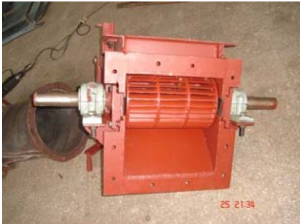
Water turbine manufactured in the EECMY-DASSC renewable energy workshop in Addis Abeba. By EECMY-DASSC renewable energy project
