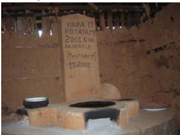
Fuel wood saving stove constructed from mud bricks with three fire/cooking places. Around 40-50% fuel wood can be saved with by using this improved stove. By Dirk Hillerkus, 2009
