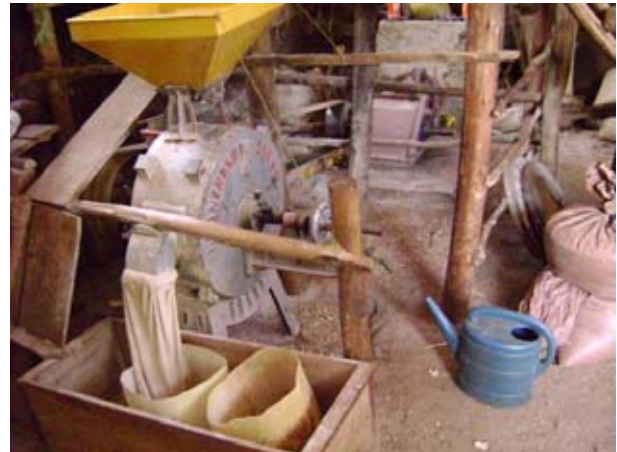
Grinding mill driven by a water turbine in Begi Gedami Synode. By Begi Gedami Synode
